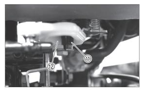
7. Check if throttle valve operates smoothly, and repeat steps1. to 6. as necessary.
