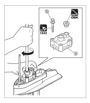
6. Feed gear oil to specified quantity. "Refer to Chapter 3."
