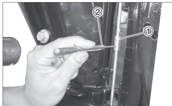
1. Remove spring pin and disconnect shift rod.
