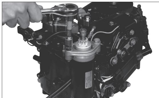
4. Install starter solenoid and PT solenoid (PT model) to solenoid stay by using bolts and nuts.
